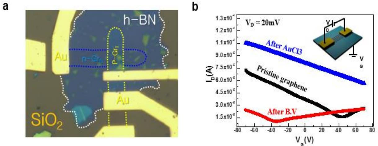
**Figure 1:** (a) A scanning electron microscopic picture of the fabricated p-type doped top graphene (p-Gr<sub>T</sub>)/ h-BN/ n-type doped bottom graphene (n-Gr<sub>B</sub>) hetero-structure. (b) Transfer curves (I<sub>D</sub>-V<sub>G</sub>) of a graphene field effect transistor (GFET) before and after doping.
