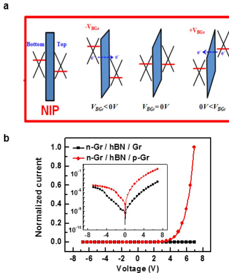
**Figure 2:** (a) Energy band diagrams under zero, reverse, and forward bias conditions. (b) Simulation results of the GBG-TDs before and after p-doping of the top graphene layer.
